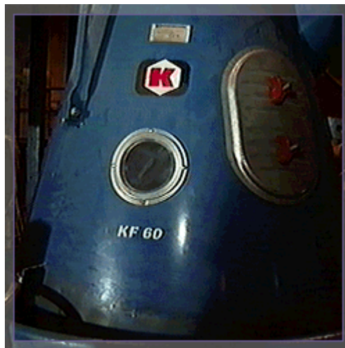
Figure 10. Air Classifier separates labels and film from the plastic flakes.
