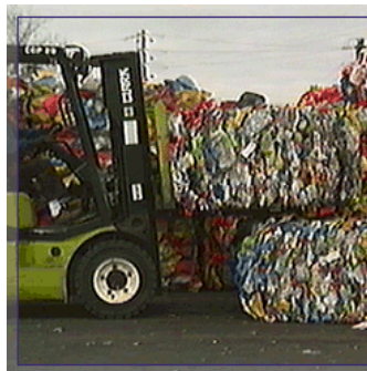
Figure 6. The sorted plastics are baled and shipped to recycling reclaimers.
