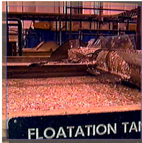
Figure 9. Float tanks are used to separate the different plastic types.
